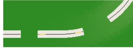
Note the yellow tips of the Quintic Easements. These tips indicate a powerful new editing feature – flexible track that maintains smooth curvature from end to end. Before completing the broken trackwork, take time to experiment with the Quintic Easements. Choose the Select Tool and point your cursor to the left end of the easement, at the yellow tip.
