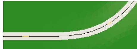
As shown above left, the left tip of the easement was dragged to the tangent track. When the tip hovers over the end of the tangent track, the tangent is highlighted in confirmation. At that point, the left mouse button is released and the easement is aligned to the tangent track.
