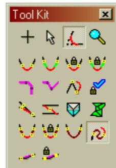
After selecting the “Connect Quintic Easement, between ends” tool, click on the end of the left track, then the end of the right track. A new piece of track is laid out between the ends, without repositioning the ends.
