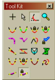
Using the tool is much the same as using the adjustable radius version discussed above. There is no need to adjust the curve using the left mouse button, though. The length of the transition curve is set to achieve the fixed radius. You can set the value of the fixed radius by pressing the button with the lock and blue check mark.
