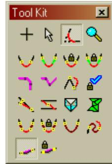
Next, point your cursor to the center of the right track segment. Press and hold the left mouse button, then move the mouse to adjust the length of the vertical easement. When you think the transition track looks reasonable, release the left mouse button to complete the connection.
